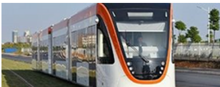
Wuhan Supercapacitor Trams, China 2016 | 21 trams, 84 cars
