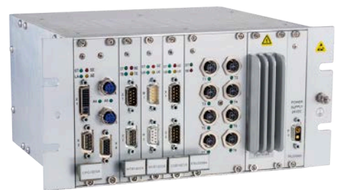
TCN Gateway with Ethernet Switches
