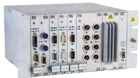
TCN Gateway with Ethernet Switches
